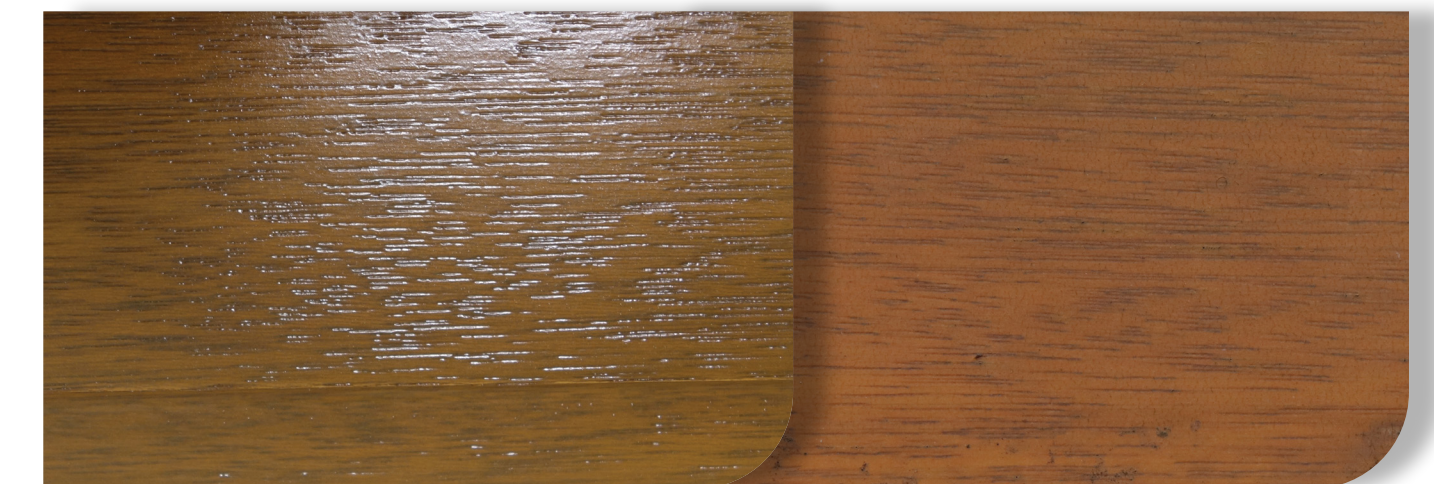
CETOL® WF 98xx before and after 4 years outdoor test
