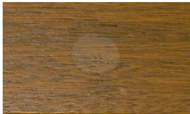
Wood treated with conventional product Result: the wood blushes, the blushing disappears after a time.
